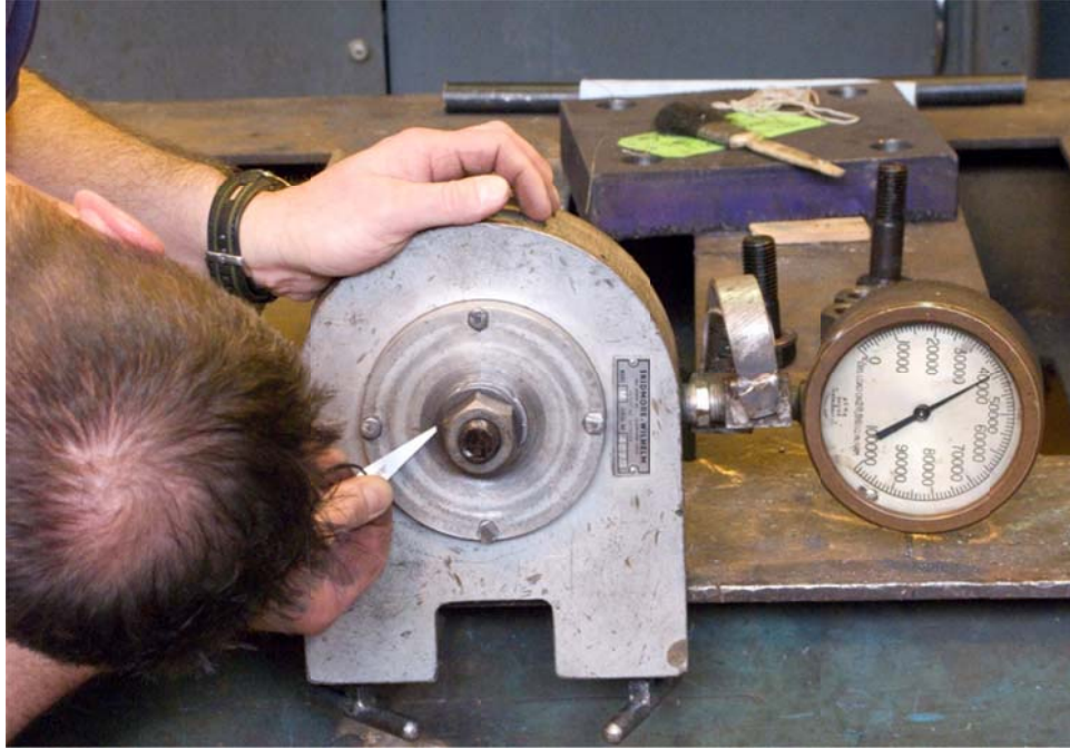
Figure 1 Periodic inspection of DTI by feeler gauge while verifying bolt tension in a Skidmore-Wilhelm tester
