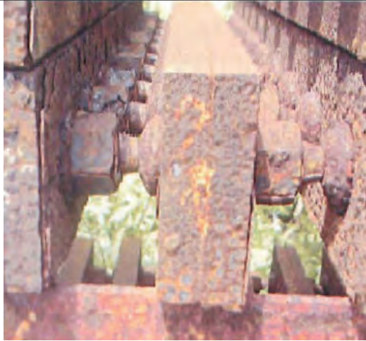
Outdoor exposure test - Okinawa
