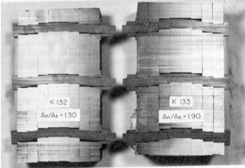
Fig. 5.33. Sawed sections of joints showing bolt bending.
