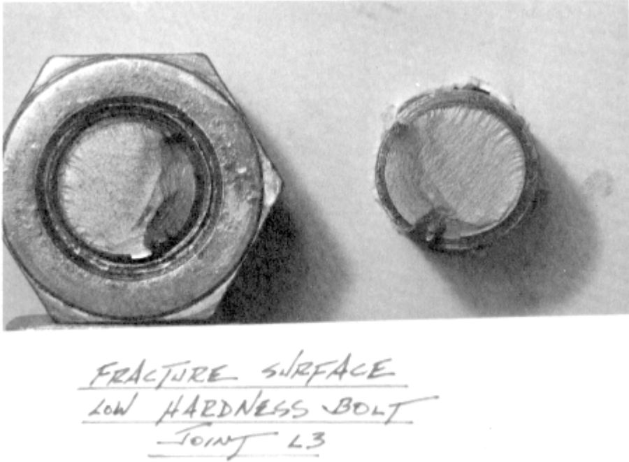
Fig. 2.7. Typical fatigue fracture surface.
