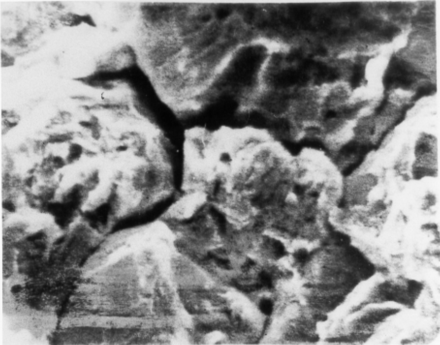
Fig 4.27. Intergranular fracture surface at the crack origin. 2000x. (Courtesy of Bethlehem Steel Corp.)
