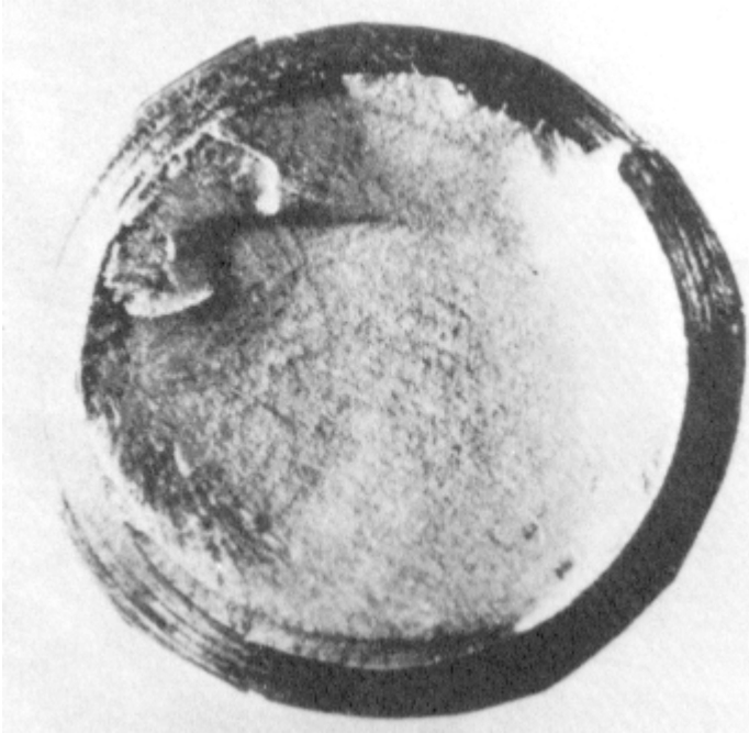
Fig 4.26. Macroscopic appearance of the crack surface (Courtesy of Bethlehem Steel Corp.)
