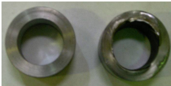
Figure 4-19: Typical Insert Before and After Testing
