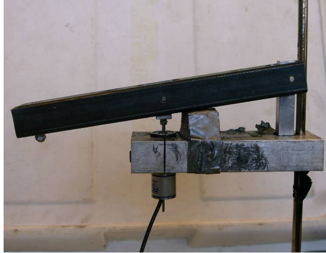
Figure 4-11: Third LVDT for Tension Testing
