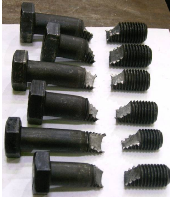
Figure 5-2: Typical Bolts Failed in Tension
