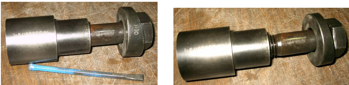
Figure 4-23: Four Complete Threads Exposed
