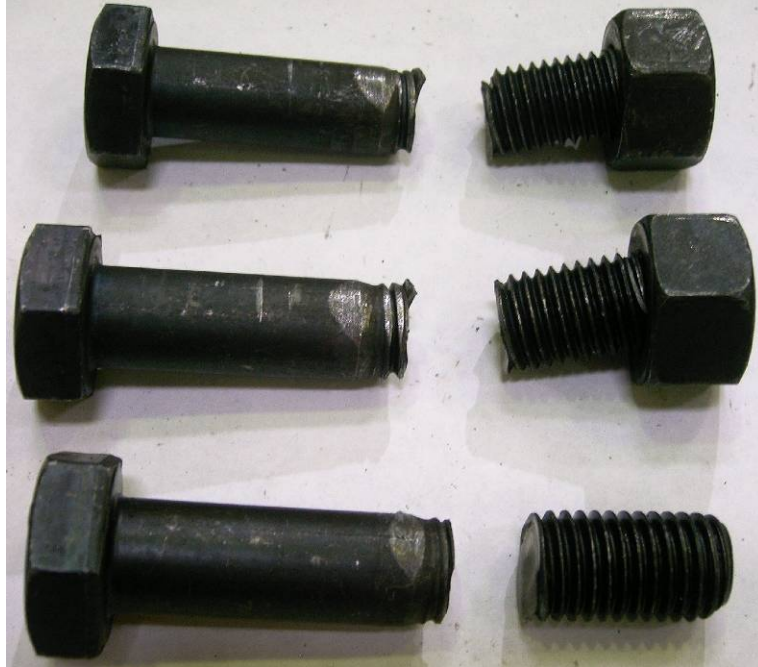
Figure 5-4: Typical Bolts Failed in Shear with the Threads Not Excluded
