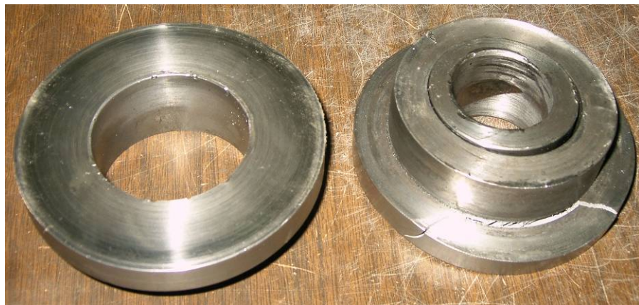
Figure 4-18: Big Inserts for 1-1/8" and 1-1/4" Bolts
