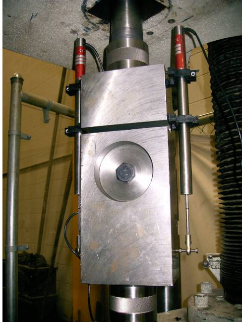
Figure 4-22: Shear Fixture Set-Up
