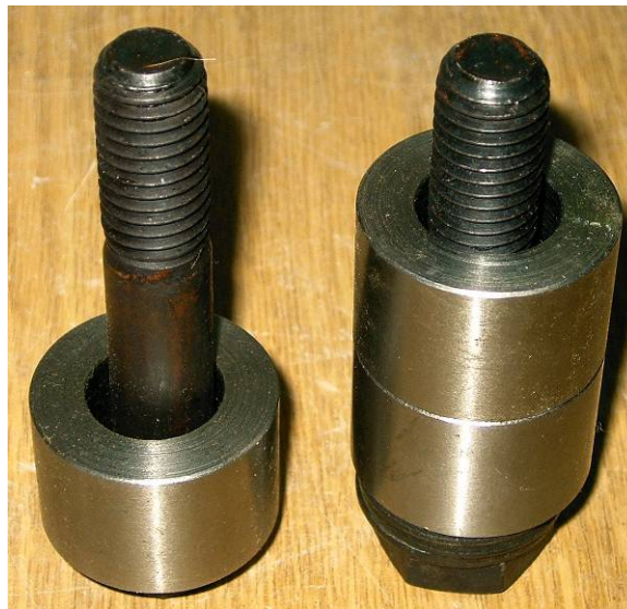
Figure 4-24: Spacers Used to Get X and N Shear Conditions
