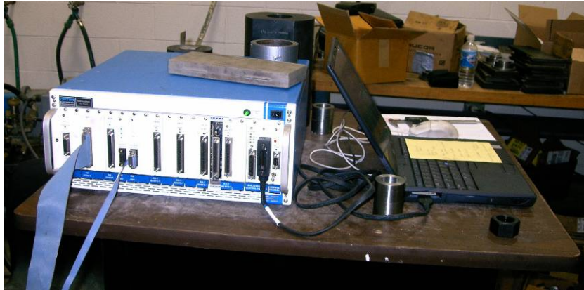
Figure 4-6: OPTIM Electronics MEGADAC with Laptop
