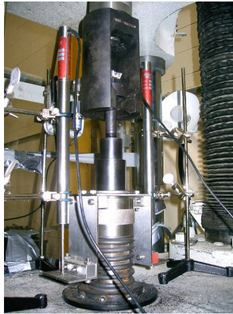
Figure 4-10: LVDT Set-Up for Tension
