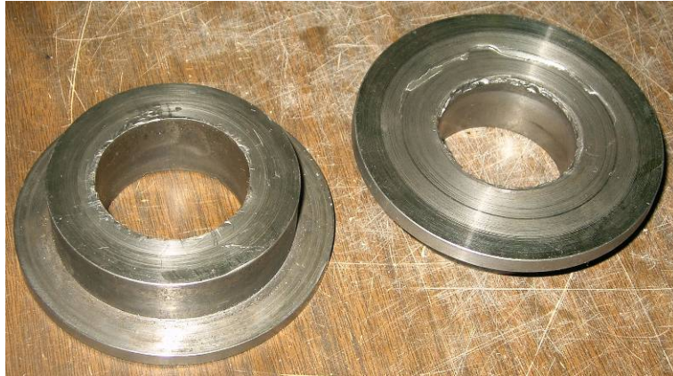
Figure 4-17: Big Insert for 7/8" and 1" Bolts
