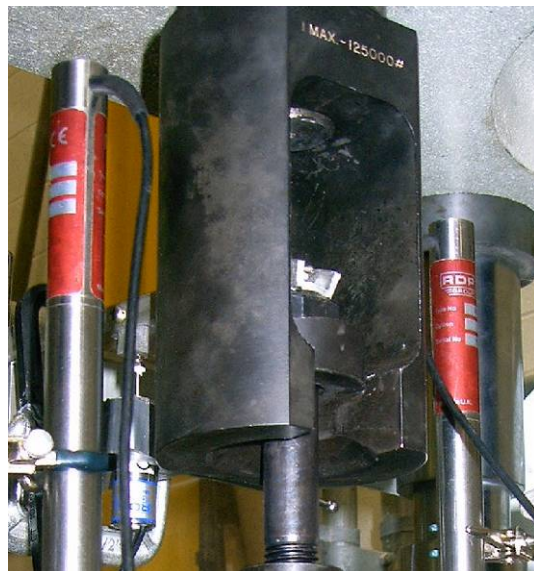
Figure 4-12: Third LVDT's Lever Arm on Bolt Head
