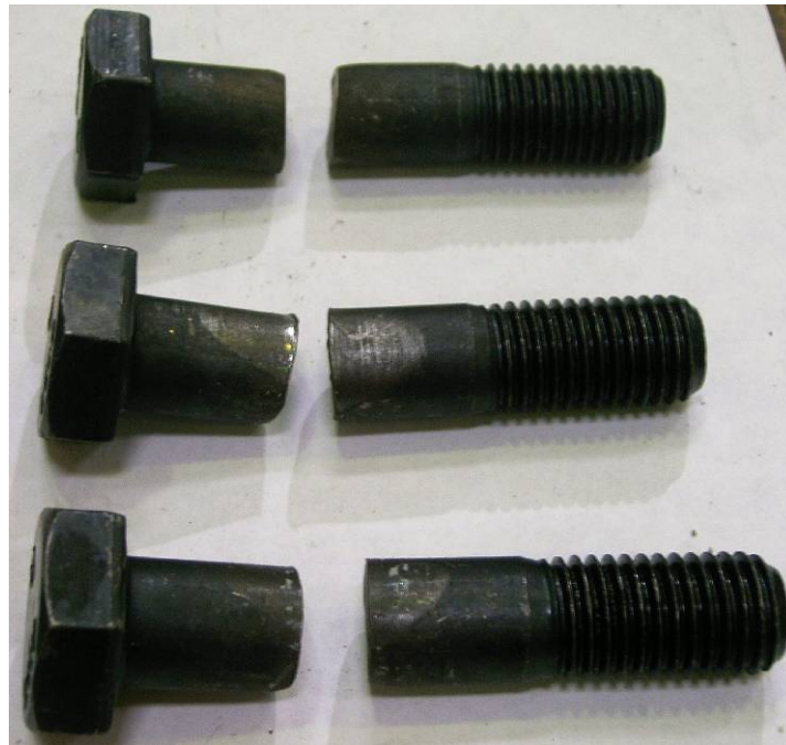
Figure 5-3: Typical Bolts Failed in Shear with the Threads Excluded
