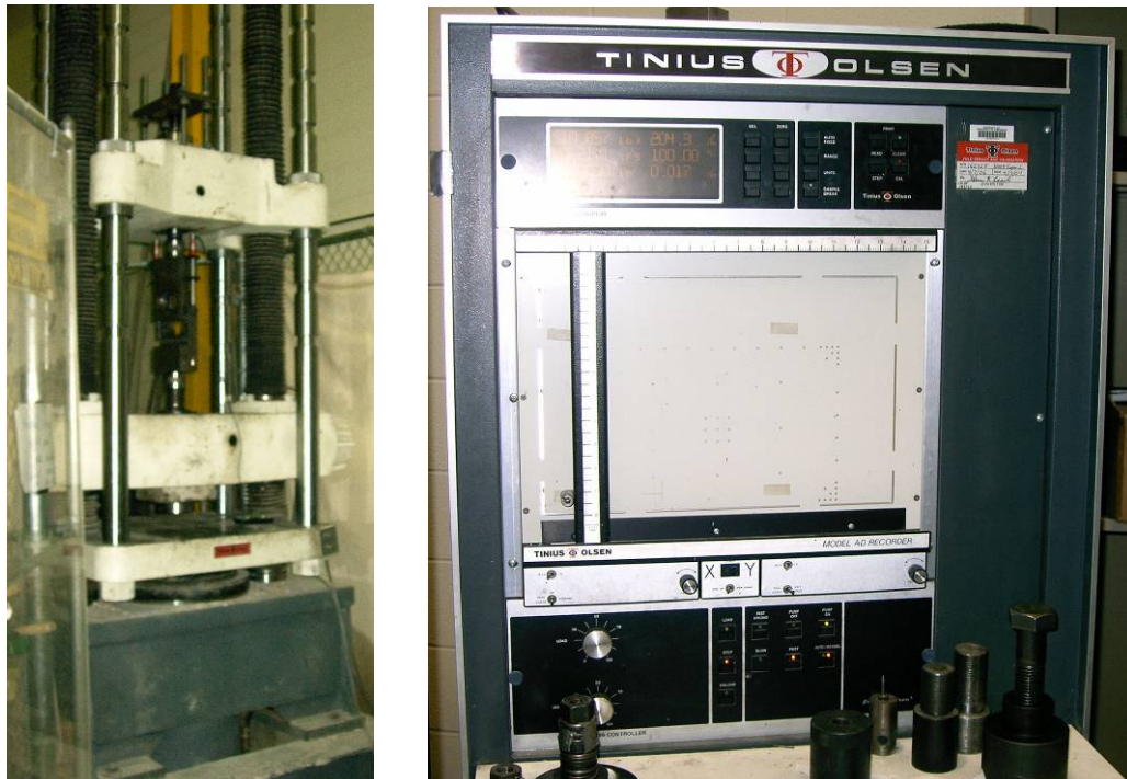
Figure 4-5: Tinius-Olsen Universal Testing Machine
