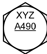
Figure 2-2: Head Marking for A490 Type 3 (RCSC 2004)
