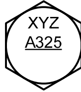
Figure 2-1: Head Marking for A325 Type 3 (RCSC 2004)
