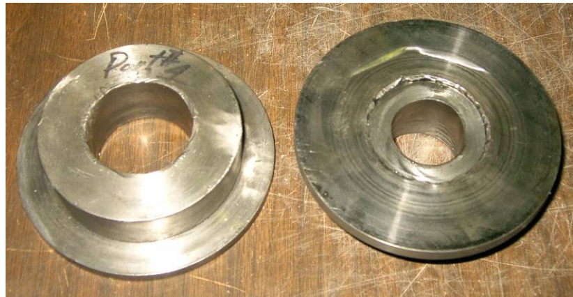
Figure 4-16: Big Insert for 5/8" and 3/4" Bolts
