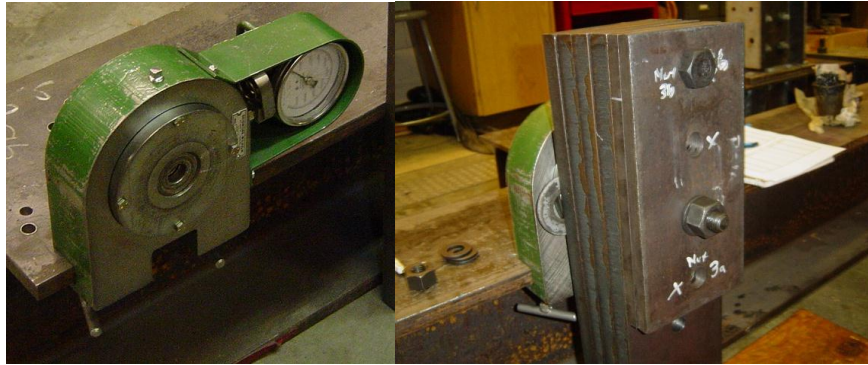
Figure 22: The Skidmore-Wilhelm bolt tensile testing device (left) and plates added to the device to accommodate the length of bolt (right).
