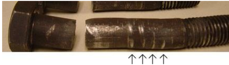
Figure 29: Impact of multi-ply fillers on a bolt and failure plane for a 4 x 0.25 in. test
