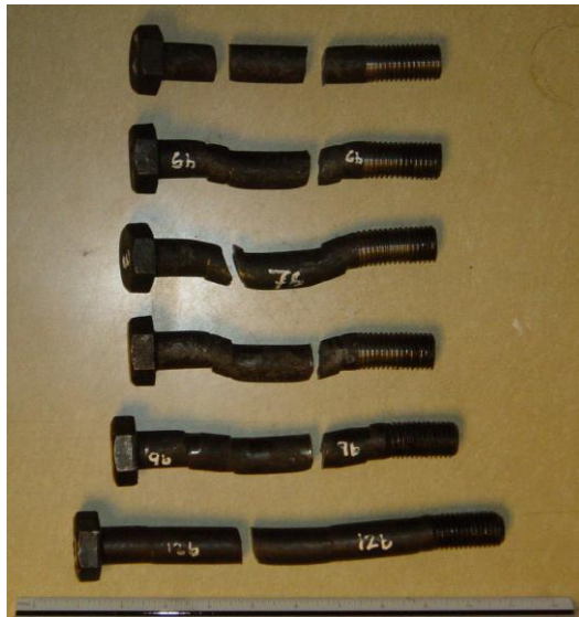
Figure 8: Sample Deformed Bolts upon Removal From Connection Assembly
