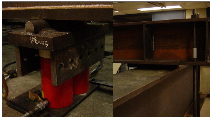
Figure 18: Applied loading points for girder splice test.
