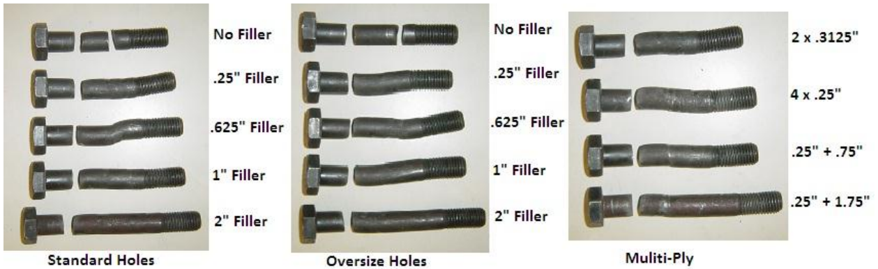
Figure 26: Examples of failed bolts for all filler thicknesses used during girder splice tests.
