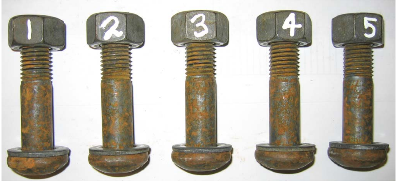
Figure 4.18 Assemblies with the bolt, nut and washer weathered separately for 2 weeks (Company A)
