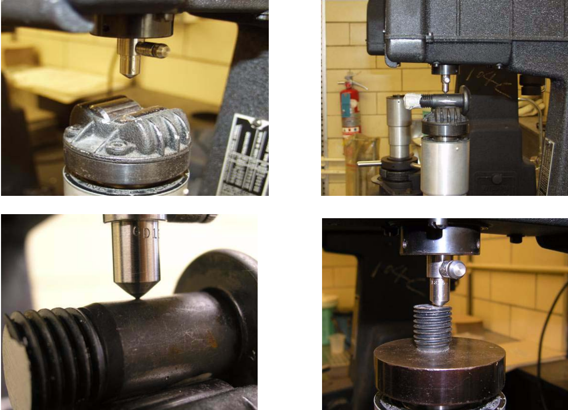
Figure 4.3 Illustration of the Rockwell hardness test
