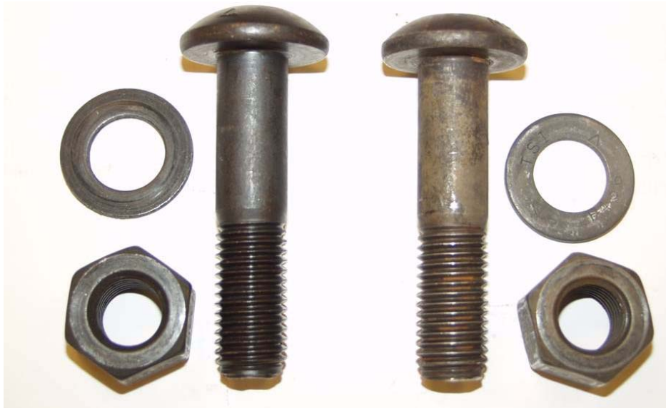
Figure 4.8 Comparison of untreated bolt (left) and bolt washed in white vinegar (right)
