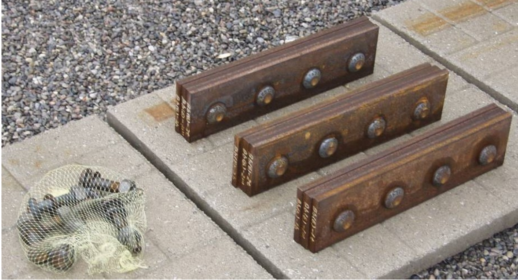
Figure 4.14 Typical weathered sample on the roof
