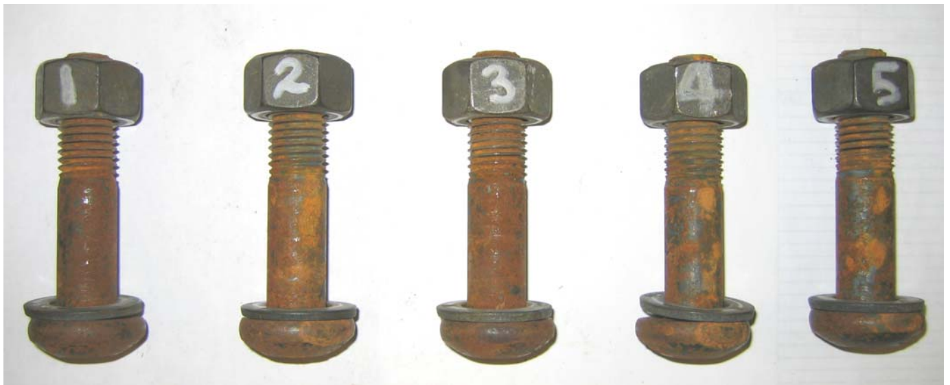
Figure 4.19 Assemblies with the bolt, nut and washer weathered separately for 4 weeks (Company A)
