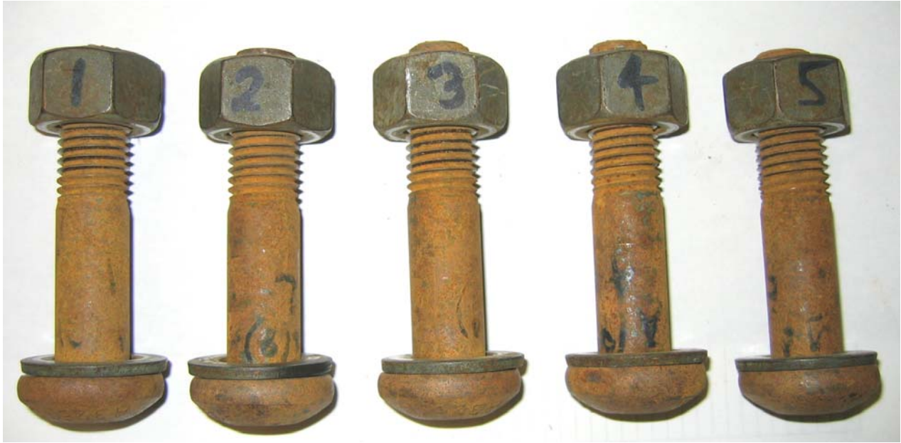
Figure 4.20 Assemblies with the bolt, nut and washer weathered separately for 8 weeks (Company A)
