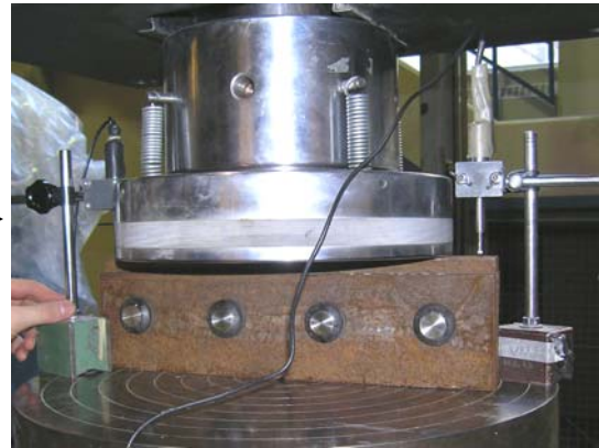
Activation of LVDT's
