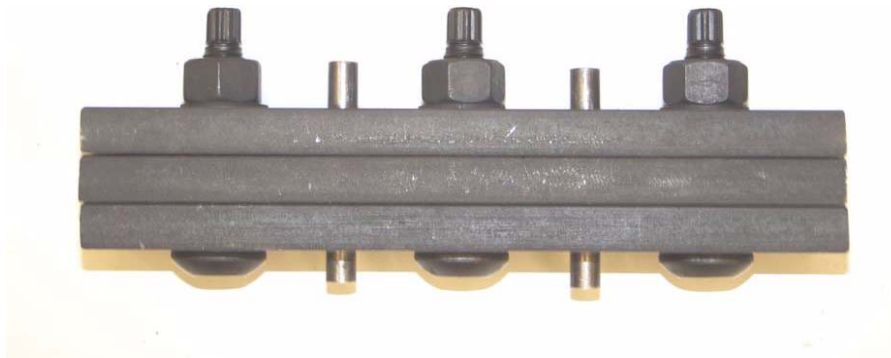
Figure 4.6 Picture of prototype 3-plate joint
