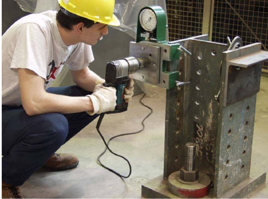
Figure 4.16 Skidmore pre-installation verification
